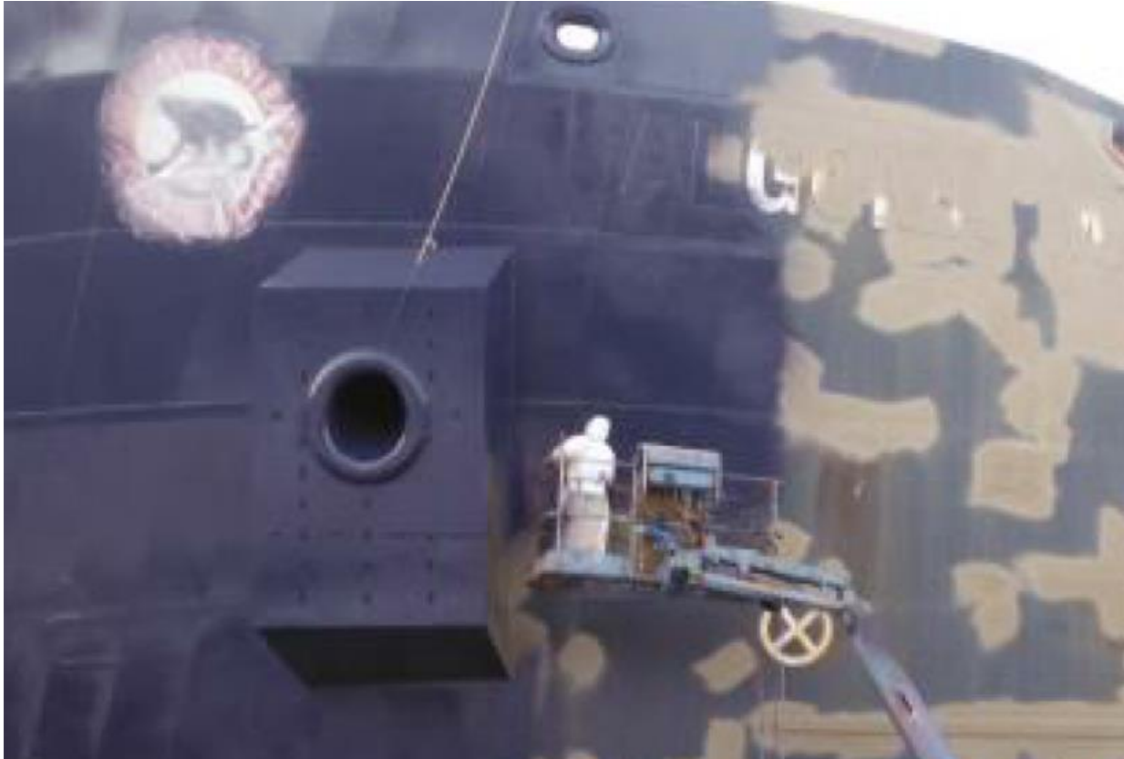
Figure 7: Hull Coating being applied.
