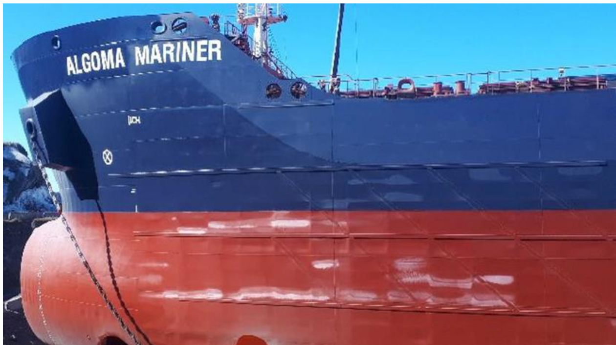
Figure 9: Side section, after hull coating refurbishment
