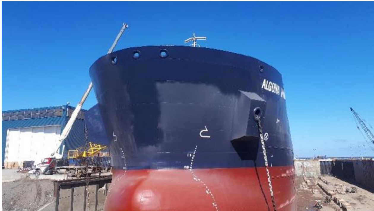
Figure 8: Bow section, after hull coating refurbishment
