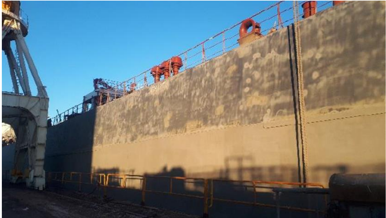
Figure 5: A portion of the hull after blasting.
