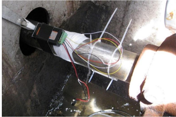
Figure A - 41 Strain Gauge Installed on Lobster Fishing Boat II
