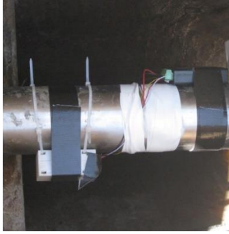
Figure A - 37 Strain Gauge Installation on Propeller Shaft
