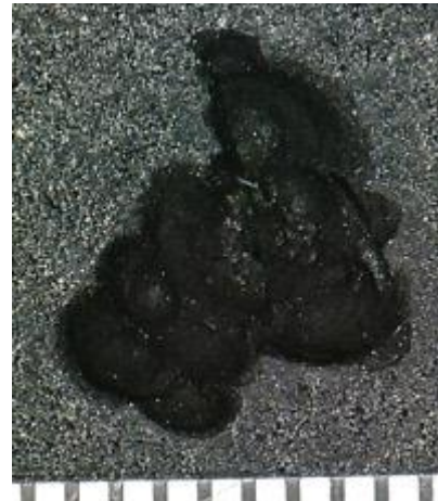
Figure 2-39: VLN on 7660 - Observed damage after 2-3 s at 0.875" offset, 90 deg.
