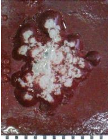
Figure 2-35: VLN on 640 - Observed damage after 15 s at 1.25” offset, 90 deg.
