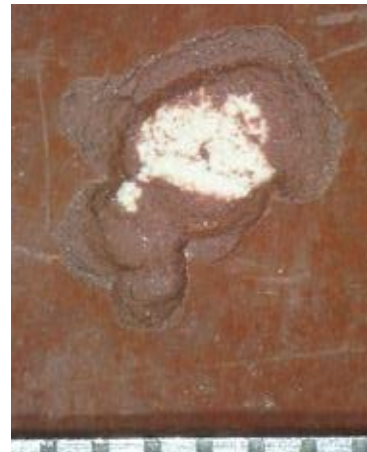
Figure 2-22: Evo2 on 640 - Observed damage after 10 s at 0.875" offset, 45 deg.
