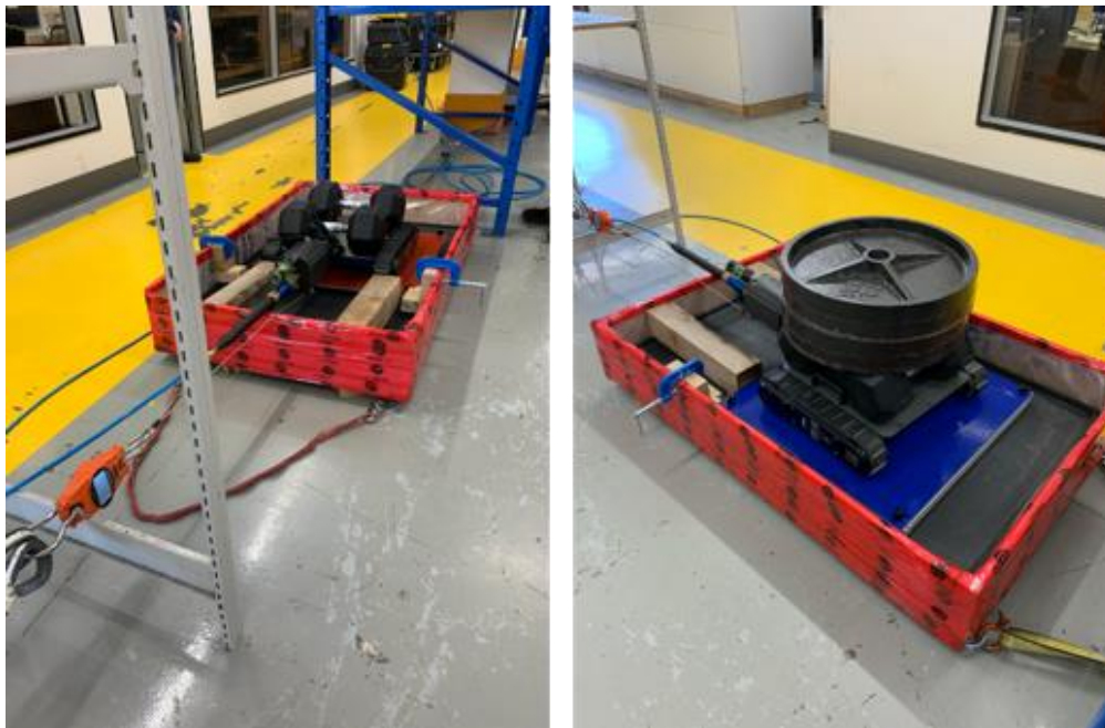
Figure 3-12: Experimental setup for testing tracks on paint. Left: crawler with 80 lb payload. Right: crawler with 260 lb payload
