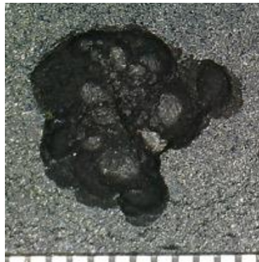
Figure 2-26: Evo2 on 7660 - Observed damage after 2-3 s at 1.25” offset, 90 deg.
