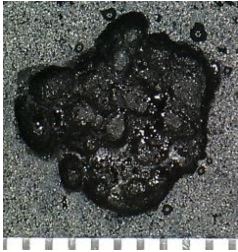
Figure 2-37: VLN on 7660 - Observed damage after 10 s at 0.875" offset, 45 deg.
