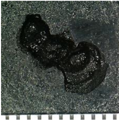
Figure 2-38: VLN on 7660 - Observed damage after 10 s at 1.25" offset, 90 deg.
