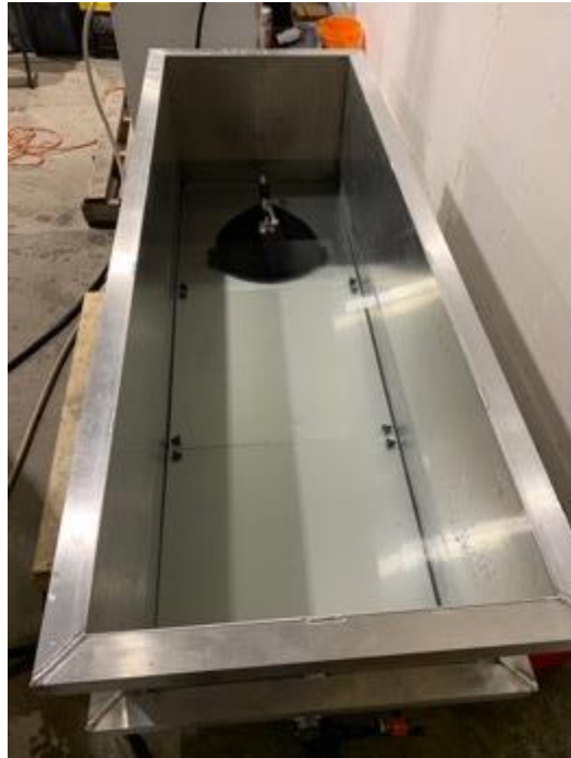
Figure 2-7: CavitCleaner Stingray placed inside test tank showing false floor
