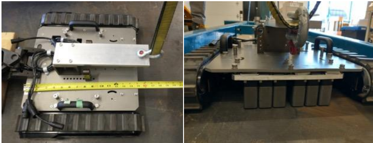
Figure 3-9. Front magnet test setup. Location of force (left), method of shimming magnets (right)
