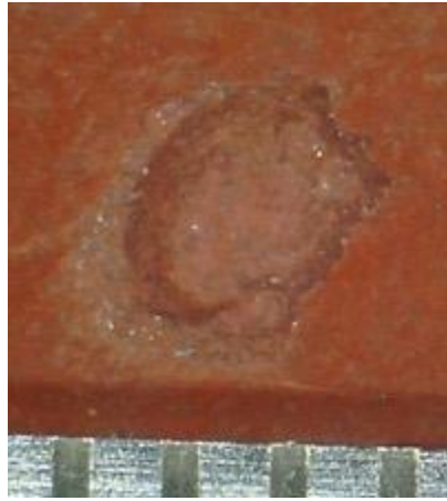
Figure 2-20: Evo2 on 640 - Observed damage after 60 s at 0.875" offset, 22 deg
