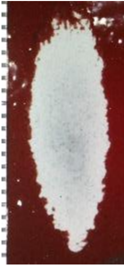
Figure 2-17: Evo2 on 1100SR - Observed damage after 2-3 s at 0.875" offset, 22 deg. (ruler scale 0.5 mm)
