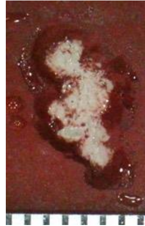
Figure 2-36: VLN on 640 - Observed damage after 2-3 s at 0.875” offset, 90 deg.
