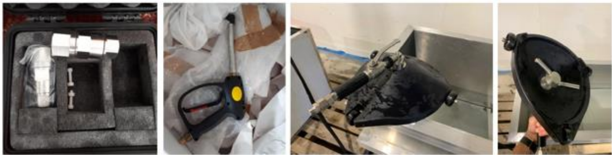
Figure 2-6: Cavijet nozzles - Left to right: VLN Nozzles, CavitaCleaner Gun, and CavitaCleaner Stingray
