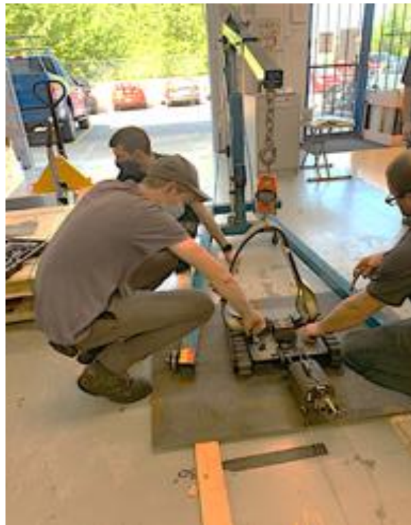
Figure 3-6: Experimental setup for magnetic strength tests
