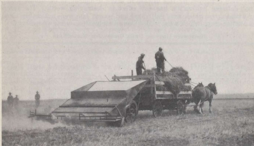
Tests of stubble-burners. A machine in operation at Swift Current.
