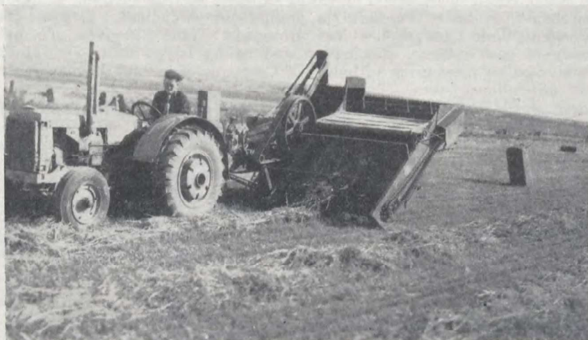
FIG. 23.—New Holland twine-type automatic tying pick-up baler at the Dominion Experimental Station, Swift Current, baling alfalfa hay.
