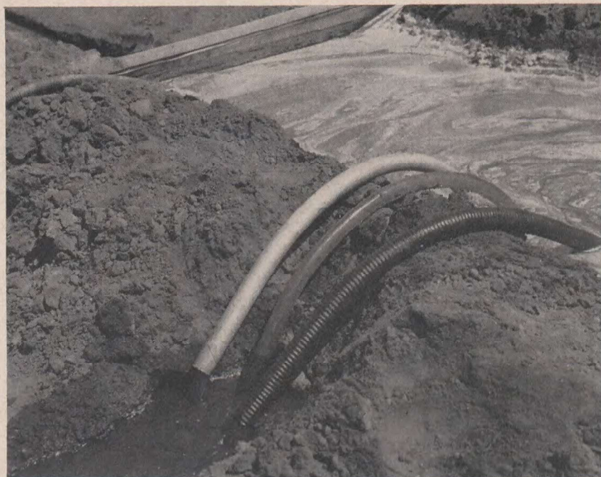
FIG. 9 Three siphon tubes in action. From left to right: aluminum, plastic, and reinforced rubber.
