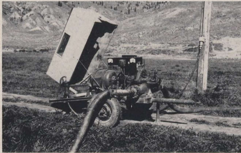
Fig. 7.—Portable electric pump used instead of buried mainline for distribution system.
