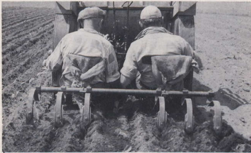
Figure 7.—Rear cultivator on a tobacco transplanter.
