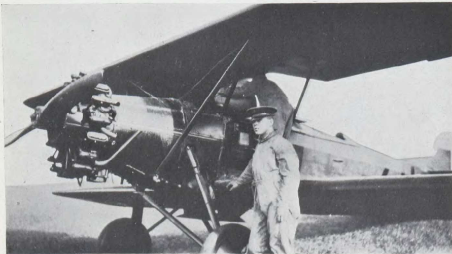
FIG. 11.—Loading the dusting plane with sulphur. Hopper capacity 600 lb.
