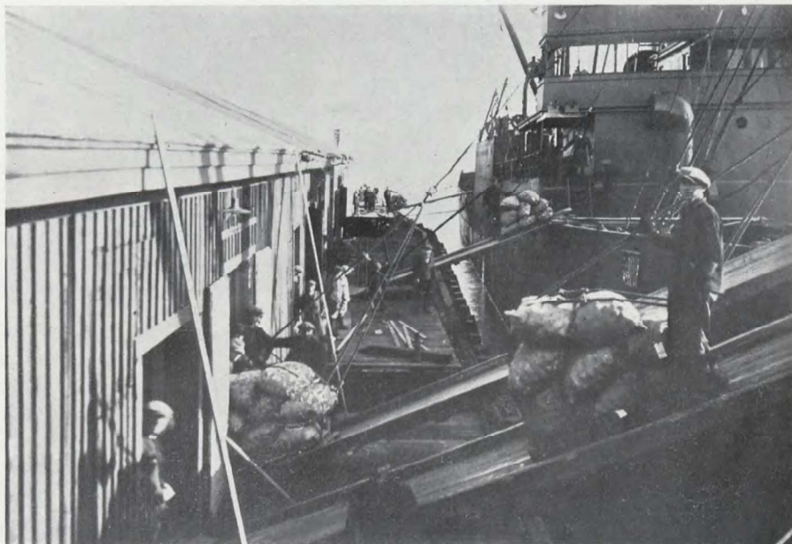
FIG. 60.—Loading cargo of certified seed potatoes at Charlottetown, P.E.I. Note arrangement of staging and slings to prevent unnecessary bruising of tubers.
