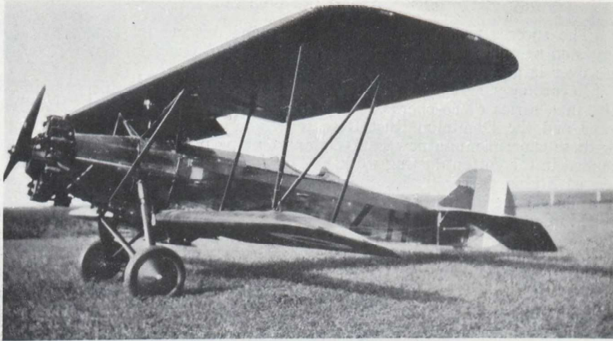
FIG. 9.—The Huff-Daland plane used for sulphur dusting operations. The dust hopper is immediately in front of the cockpit from which the machine is controlled.
