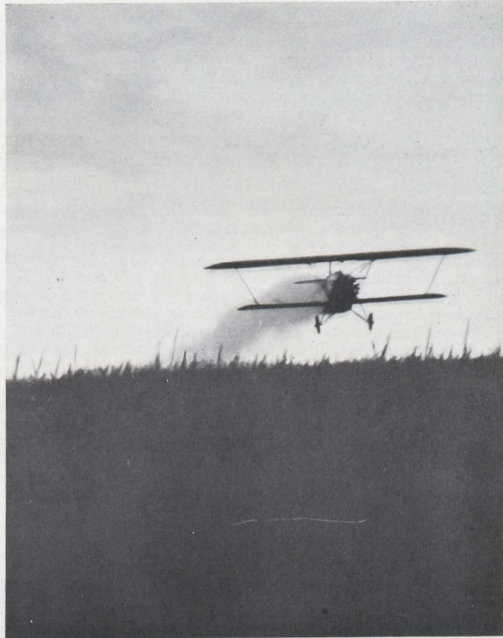
FIG. 12.—Dusting plane approaching the camera, showing the downward trend of the dust cloud.
