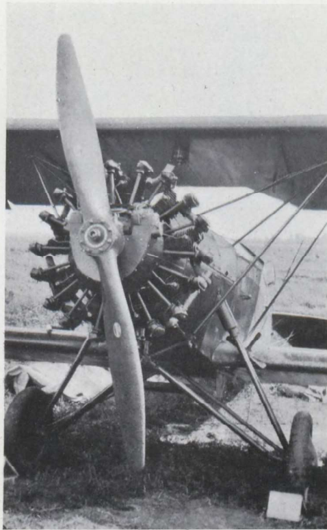
FIG. 10.—Huff-Daland plane. The distributor through which the dust is discharged is shown projecting below fusilage. Dust delivery is controlled by the pilot. The small propeller turns the agitator inside of the hopper.
