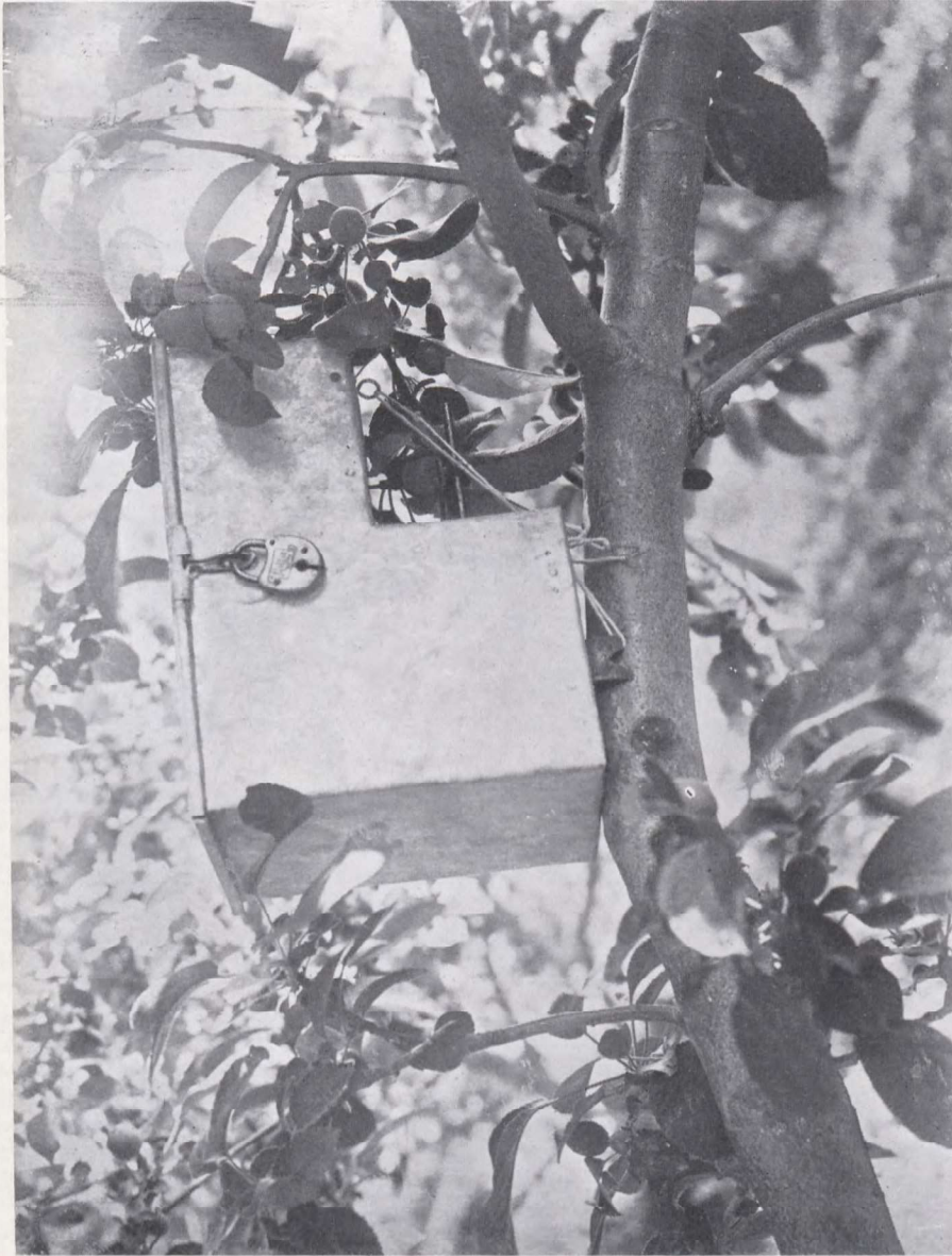
FIG. 46.—An apple-measuring machine in position on the limb. The apple being measured can be noticed just underneath the raised end of the measuring box.
