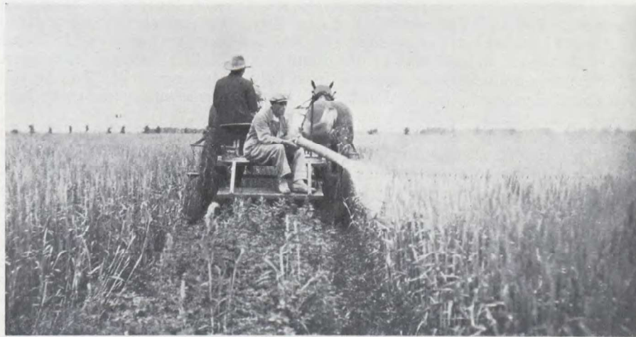
FIG. 7.—Horse-drawn traction dusting machine (Niagara Traction Crop Duster C-26-P) in operation. A cloud of dust is discharged through a flexible delivery tube, 5 inches in diameter.
