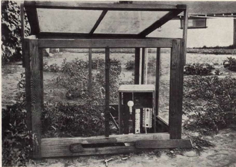
FIG. 38.—Glass cage set up in position over one-half of a tomato plant to expose it to high temperatures during the day, showing arrangement of the maximum and minimum thermometer, hygrometer, soil thermometer, and atmometer used in the tests. Note the untreated, check portion of the vine at the left.
