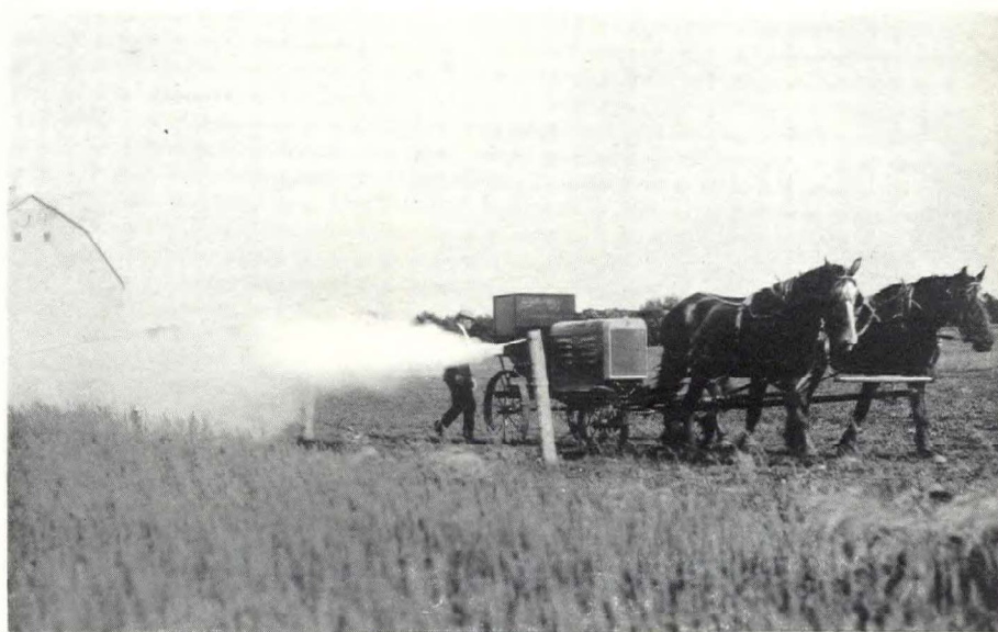
FIG. 17.—Horse-drawn power dusting machine (Shunk duster) in operation. The dust is forcibly discharged through a wide delivery tube.
