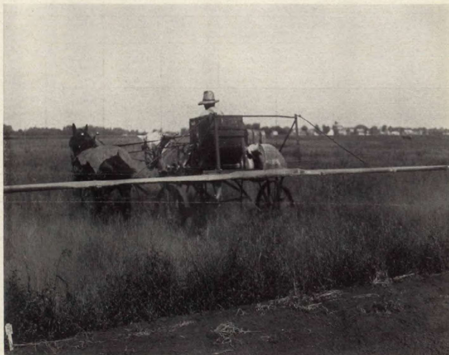
FIG. 18.—Horse-drawn power duster (Niagara Aero duster) with an attached boom distributor. This machine is capable of dusting a strip 30 feet wide.
