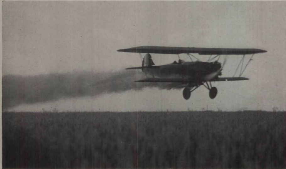
FIG. 5.—Dusting plane in operation, showing behaviour of the dust after being discharged from the hopper. The machine is flying at an altitude of from 10 to 15 feet.
