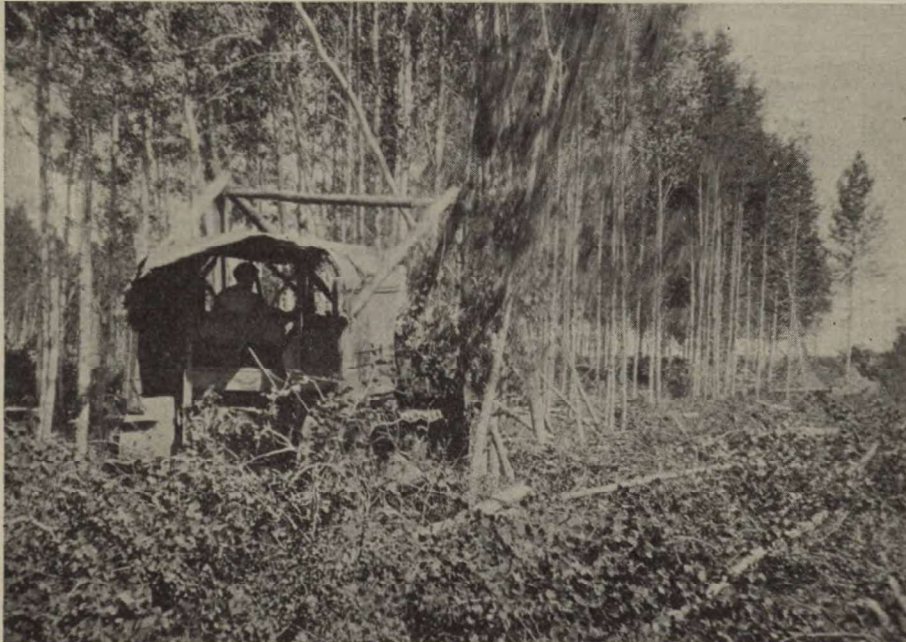
A 60-horsepower caterpillar brush cutter at work. This machine will clear 10 to 12 acres of brush land per day, and has been partly responsible for the increased area under cultivation in the park belt.
