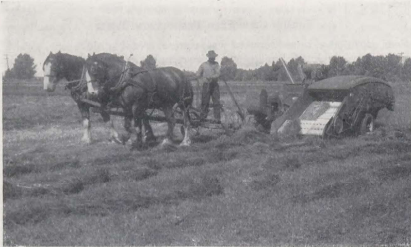
Fig. 17.—Threshing alsike clover windrows with a small pick-up combine. A combine equipped with an auxiliary motor is preferred to one operated from a power take-off. It enables a uniform cylinder speed to be maintained regardless of the speed of forward travel.
