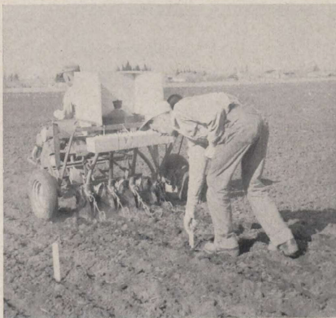
FIG. 2—Four-row power plot seeder in operation at Lacombe. With this unit two men can seed 480 rod rows per hour.
