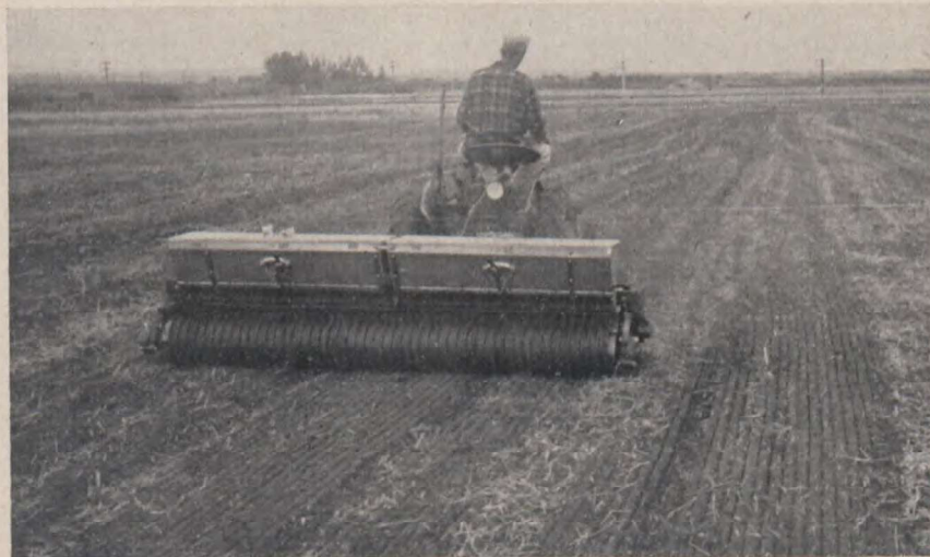
FIG. 5—This type of combination seeder and packer gives a firm seedbed, uniform distribution of seed, and shallow seeding, thereby eliminating much of the risk involved in establishing good stands of grasses and legumes.
