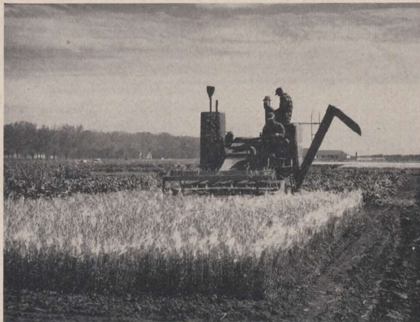
FIG. 1—The self-propelled combine has proved to be an excellent harvesting implement for securing accurate yields on medium to large grain plots.
