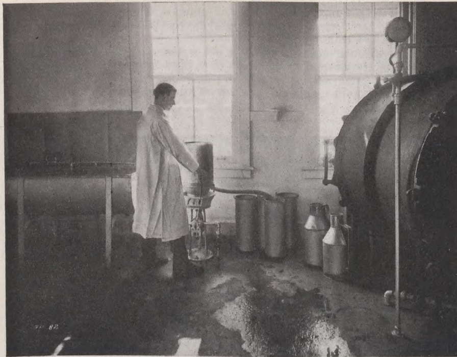
Washing and steaming utensils prior to sterilization in the large autoclave to the right.
