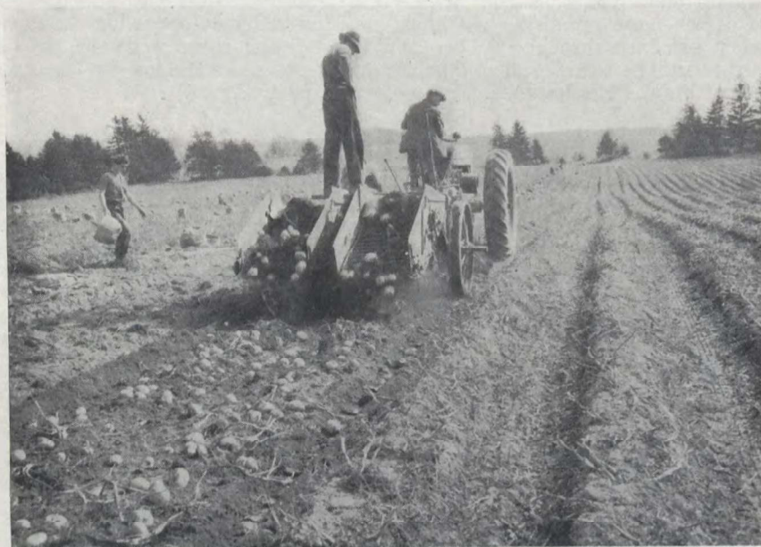
Figure 21—Two-row potato digger.
