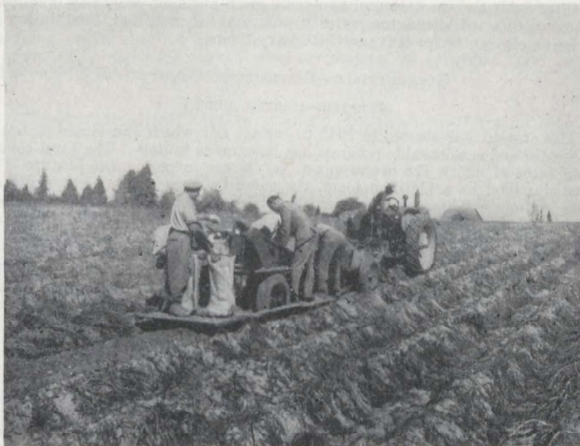
Figure 22—Potato digger and picker, Keswick, N.B.
