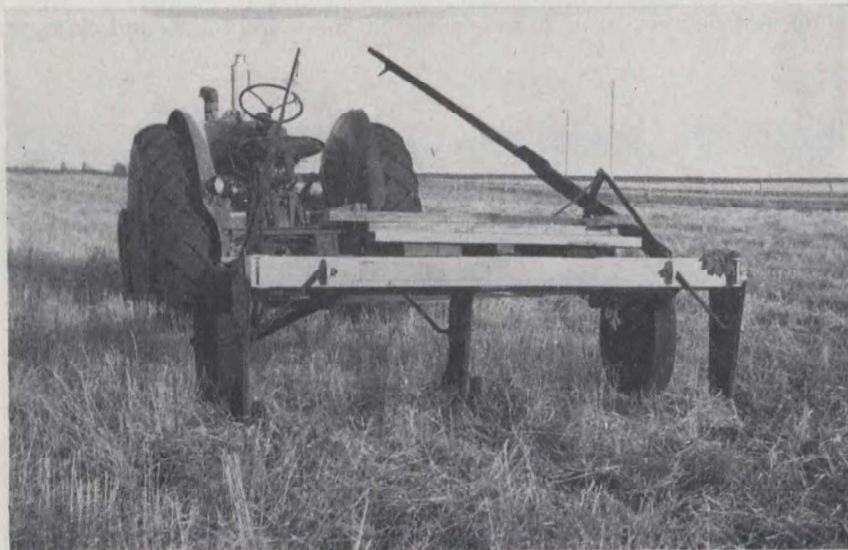
FIG. 10.—The blade cultivator anchors the trash cover and is a most useful machine for moisture conservation and soil drift control.
