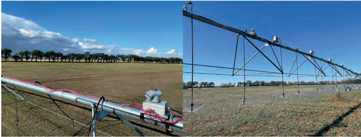
Figure 44. Automated Site Specific Variable Rate Irrigation (SS-VRI) sensors and valves mounted on a centre pivot irrigation system (InteliRain 2023)
