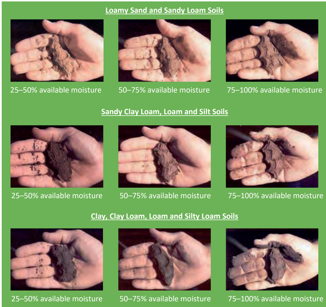
Figure 15. Available soil moisture ranges for various soil textures using hand feel method (NRCS).
