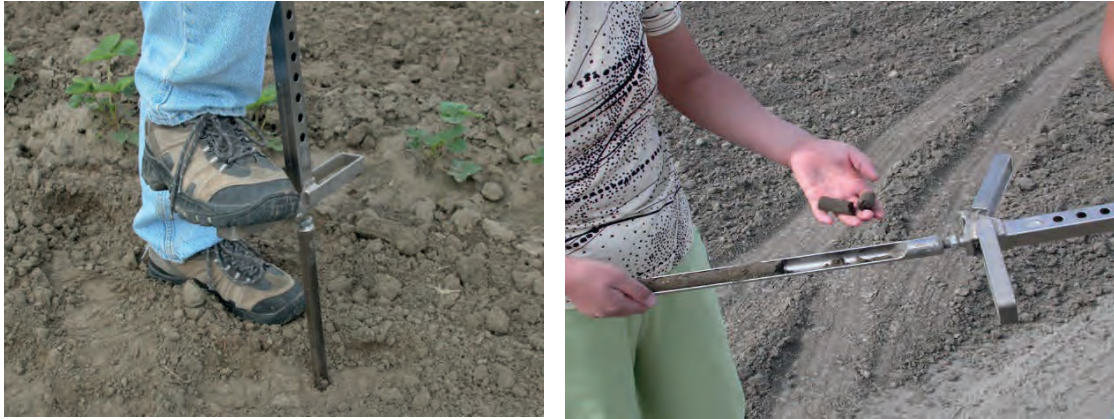
Figure 7. Soil sample collection using a JMC Backsaver soil core sampler.
