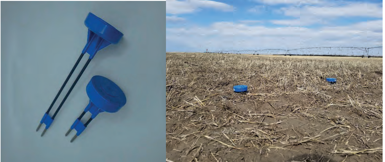
Figure 19. Example of TDR probes with built-in data transmission capacity (left) installed in irrigation field (right).
