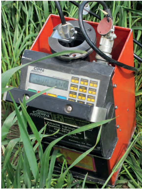
Figure 23. Neutron Probe Soil Moisture Sensor (L. Hingley, Government of Alberta)
