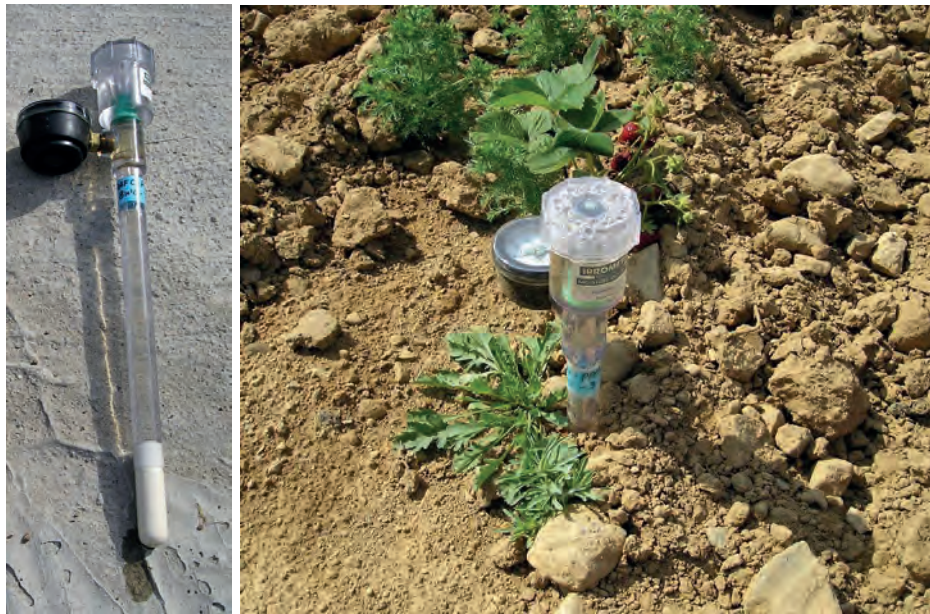
Figure 16. Tensiometers measure soil tension which can be translated into soil moisture content.
