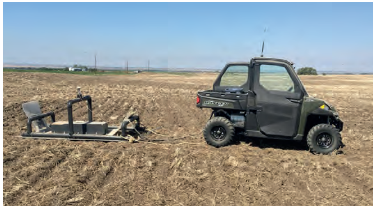
Figure 39. Electromagnetic (EM) sensor on field sled for conducting EM and topographical surveys.
