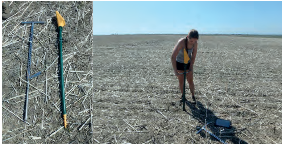
Figure 21. Example of a tube style capacitance probe (left) being installed in irrigation field (right).
