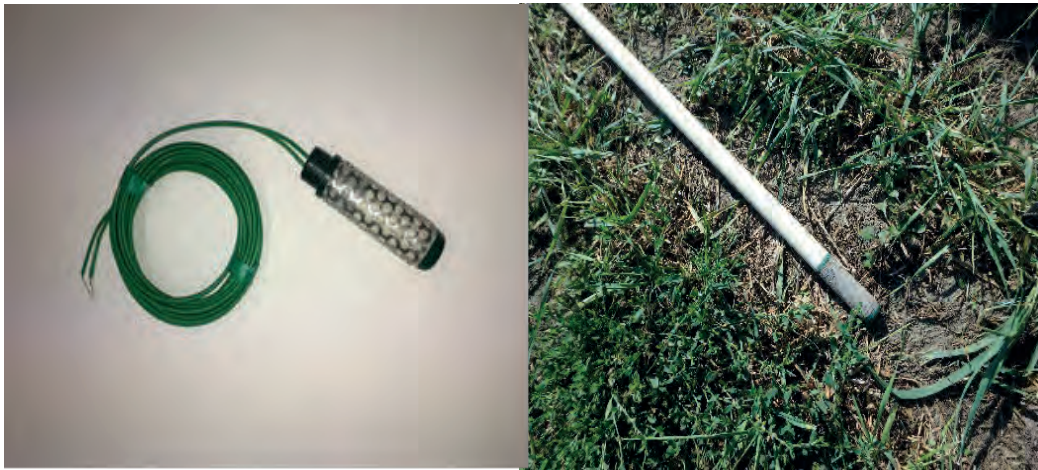
Figure 18. Example of a granular matrix block (left) attached to a PVC access tube (right).
