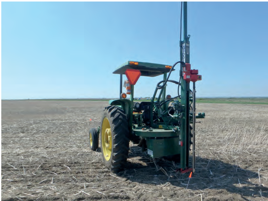
Figure 8. Hydraulic soil sampler/coring machine mounted to tractor.
