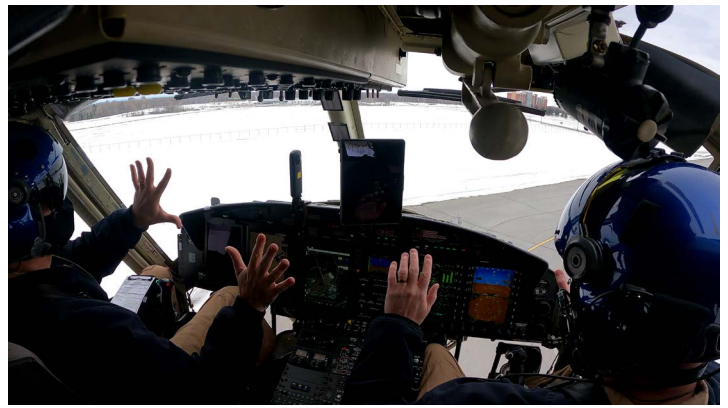
Cockpit view of the NRC's Bell 412 Advanced Systems Research Aircraft with test pilots supervising the autonomous landing in between obstacles.
