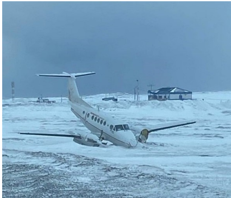
Figure 3. The occurrence aircraft after the runway excursion, stopped with the nose down (Source: Keewatin)
