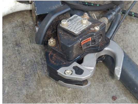
Figure 6. Cargo hook from the occurrence helicopter in the open position, after the mechanical (cable) release lever had been actuated (Source: McLarens Aviation)
