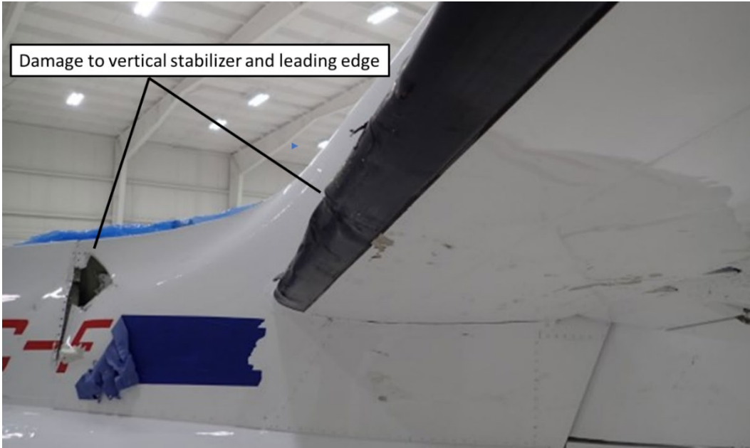
Figure 3. Photo showing the damage to the vertical stabilizer and leading edge of the left horizontal stabilizer (Source: TSB)
