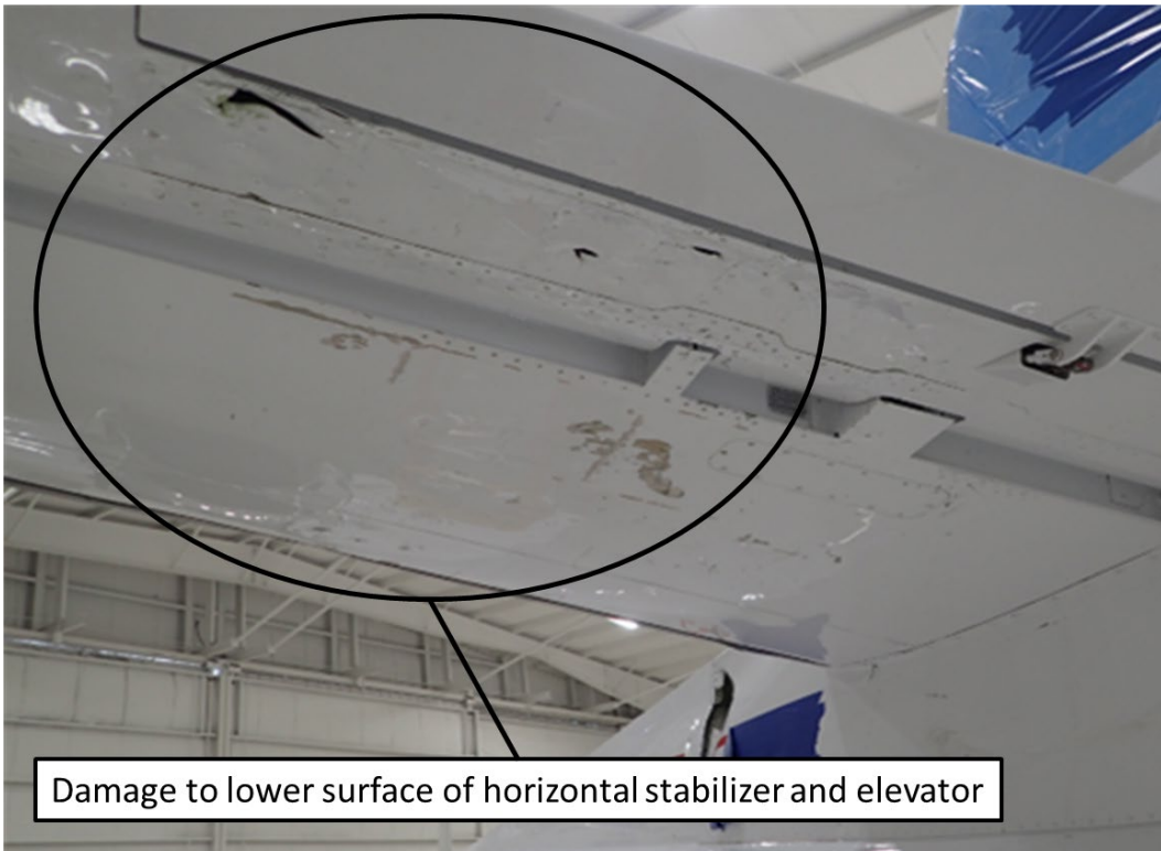
Figure 4. Photo showing damage to the lower surface of the left horizontal stabilizer and elevator (Source: TSB)
