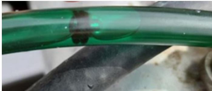
Figure 5. Electrical grommet found in fuel return line (Source: TSB)
