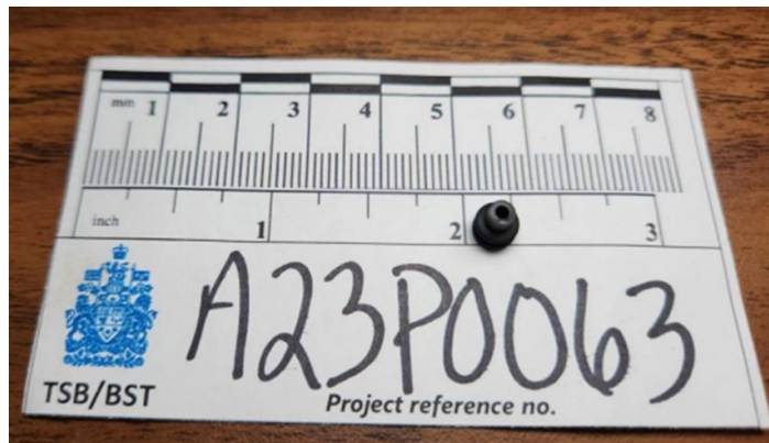
Figure 5. Electrical grommet found in fuel return line (Source: TSB)
