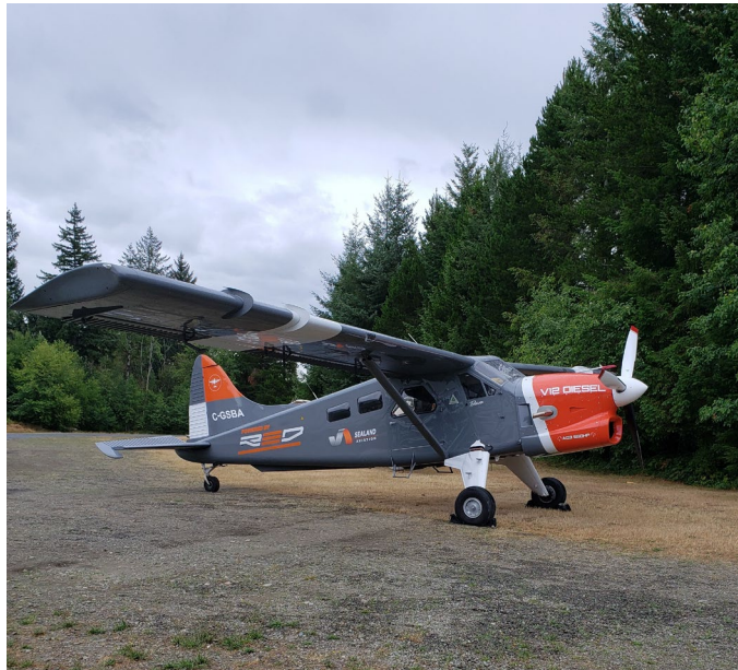
Figure 2. Occurrence aircraft equipped with the RED A03-005 engine (photo taken before the occurrence) (Source: Third party, with permission)
