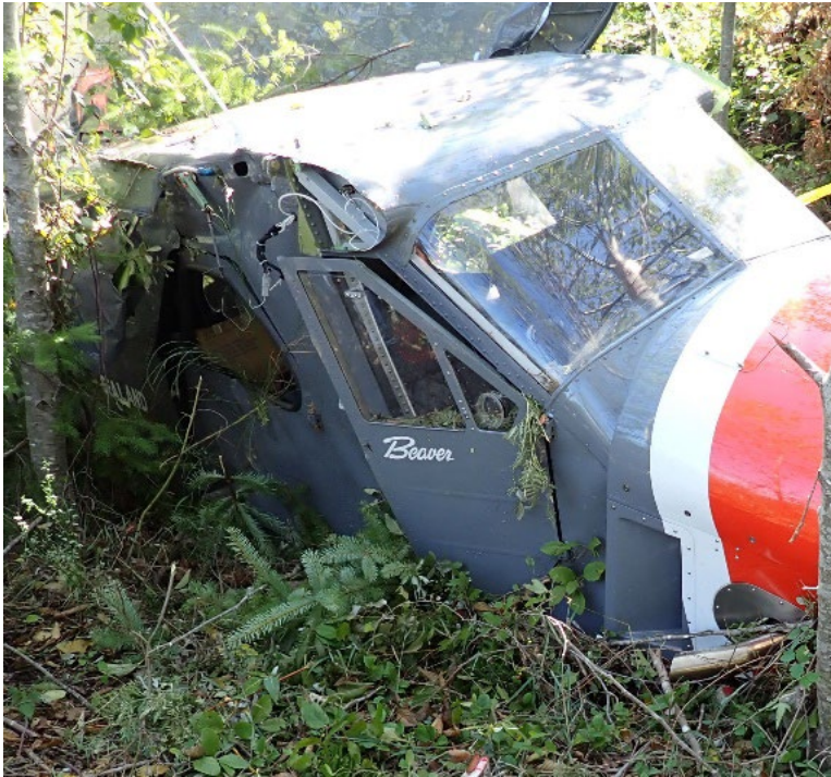
Figure 5. Accident site, showing right cockpit door obstructed by terrain (Source: TSB)
