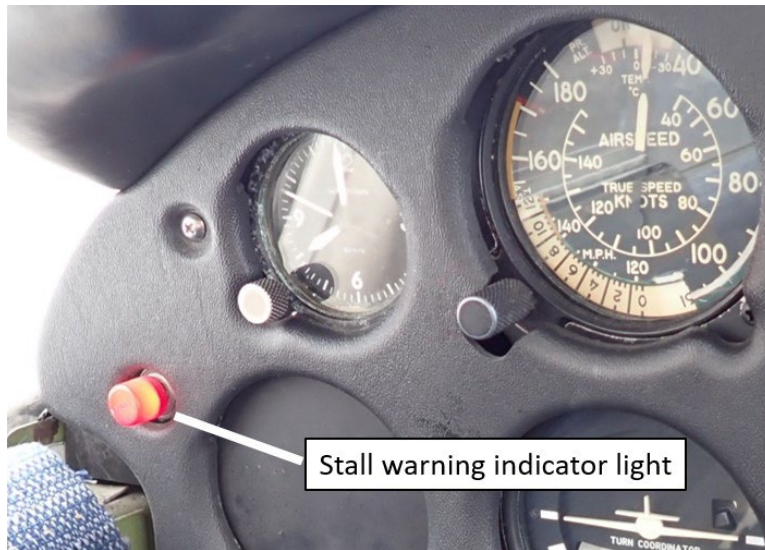
Figure 3. Illuminated stall warning light in an aircraft similar to the occurrence aircraft type (Source: TSB)
