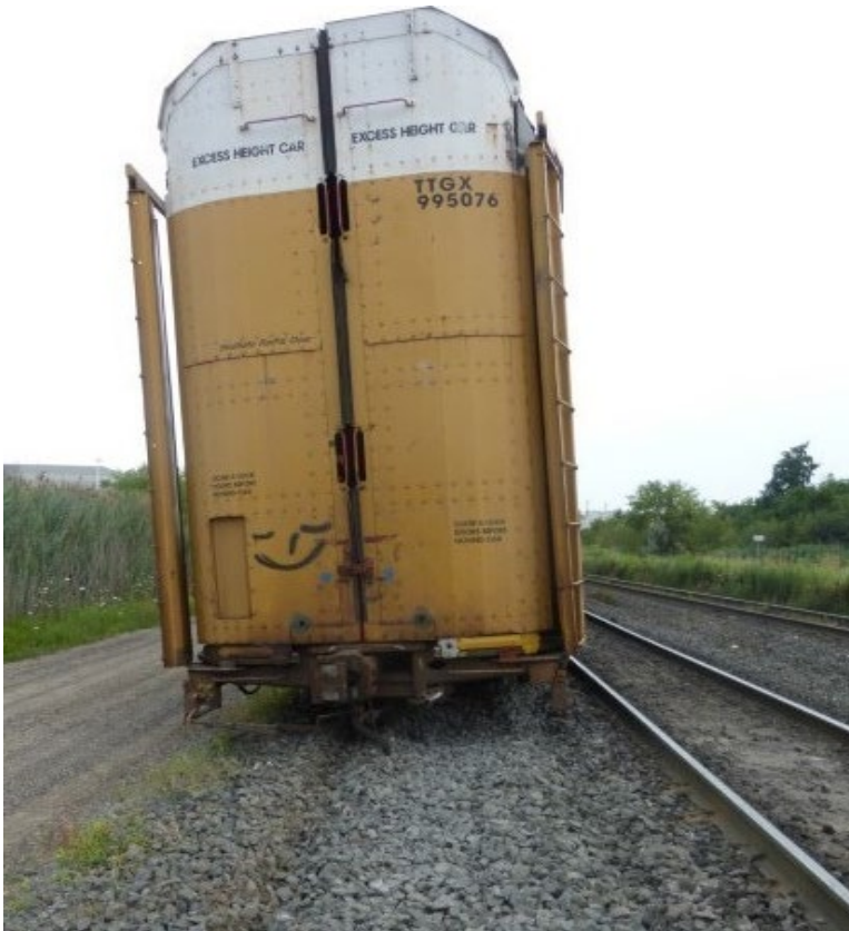
Figure 5. Trailing B-end truck of 26th car TTGX 995076 derailed; A-end truck remained on the rails (Source: TSB)
