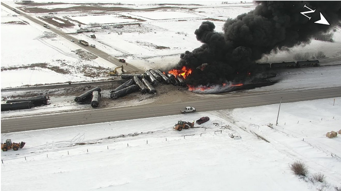
Figure 2. Aerial view of the derailment site, taken at 1300 on 06 February 2020, showing derailed tank cars, several of which are engulfed in a large fire (Source: Humboldt fire department)
