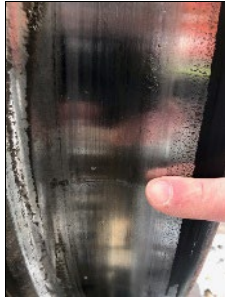
Figure 4. Impact mark on the tread of a wheel from the north side of car CBTX 721371 (line 28) (Source: Canadian Pacific)
