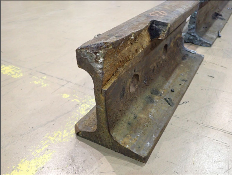
Figure 5. West end of the recovered plug rail, showing impact mark and missing rail head (Source: TSB)
