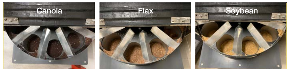
Figure 4 Rotary divider modified with a metal collar that minimizes grain loss in subsamples.
