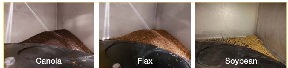
Figure 3 Accumulation of grain in the housing of a rotary sample divider that is lost from subsamples.
