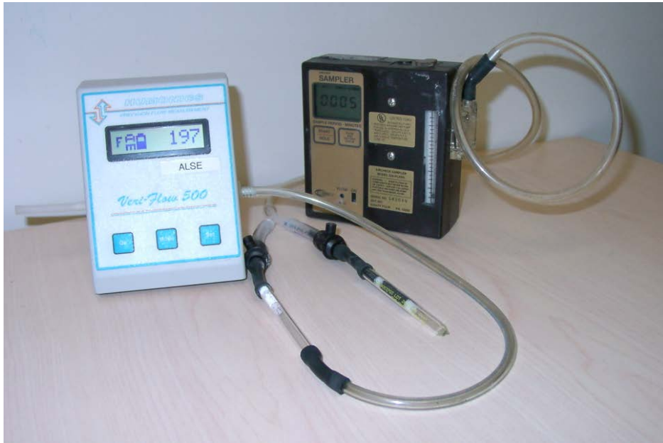
FIGURE 4: Flow Rate Calibration of Sorbent Tubes (courtesy ALS, Vancouver, BC)
