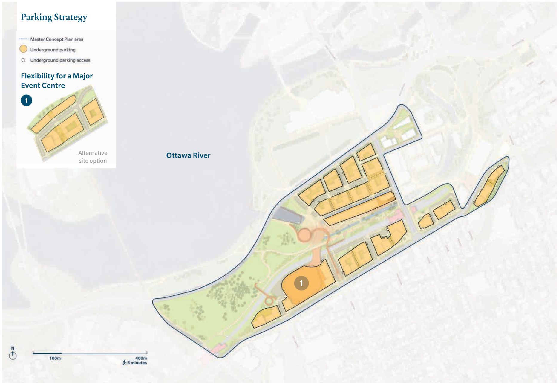
Figure 32 The LeBreton Flats Master Concept Plan parking concept reduces the amount of surface parking to encourage a vibrant public realm by locating the majority of parking underground.
