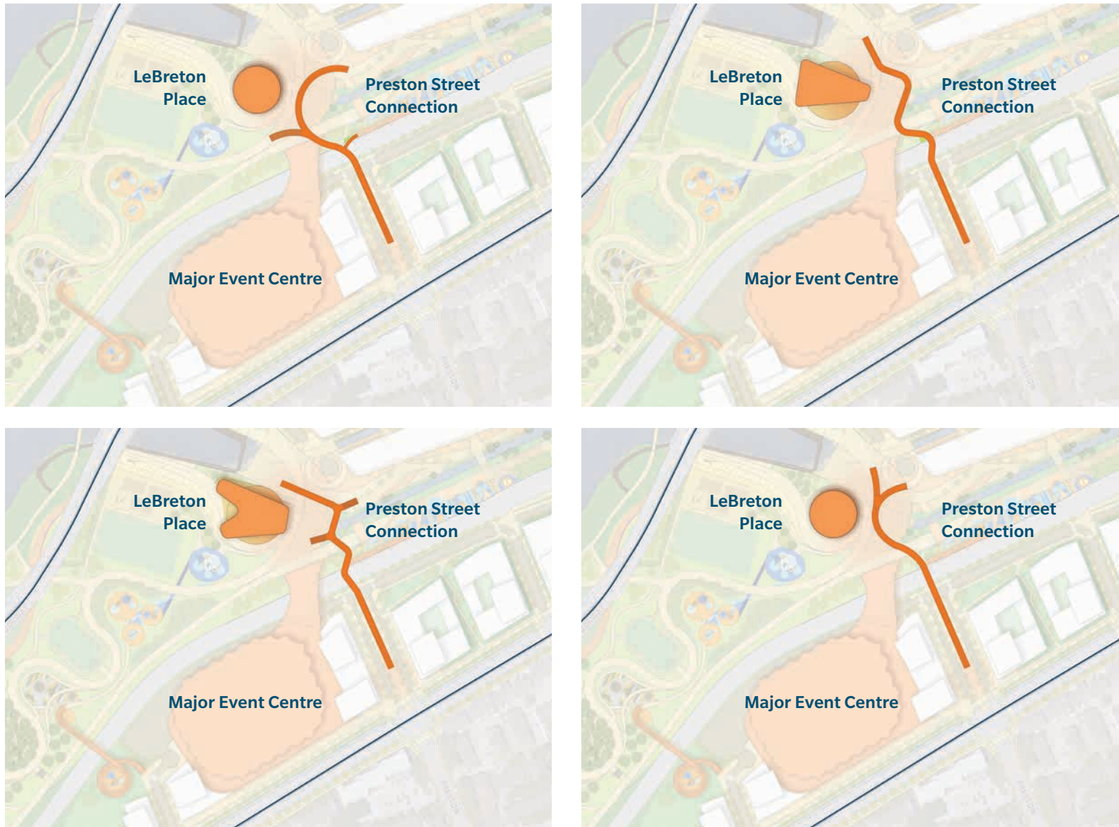
Figure 27 The configuration of a pedestrian/cycling bridge in the Preston Street corridor will be subject to a future design process. These images illustrate a number of potential options for the configuration of a bridge in this location.
