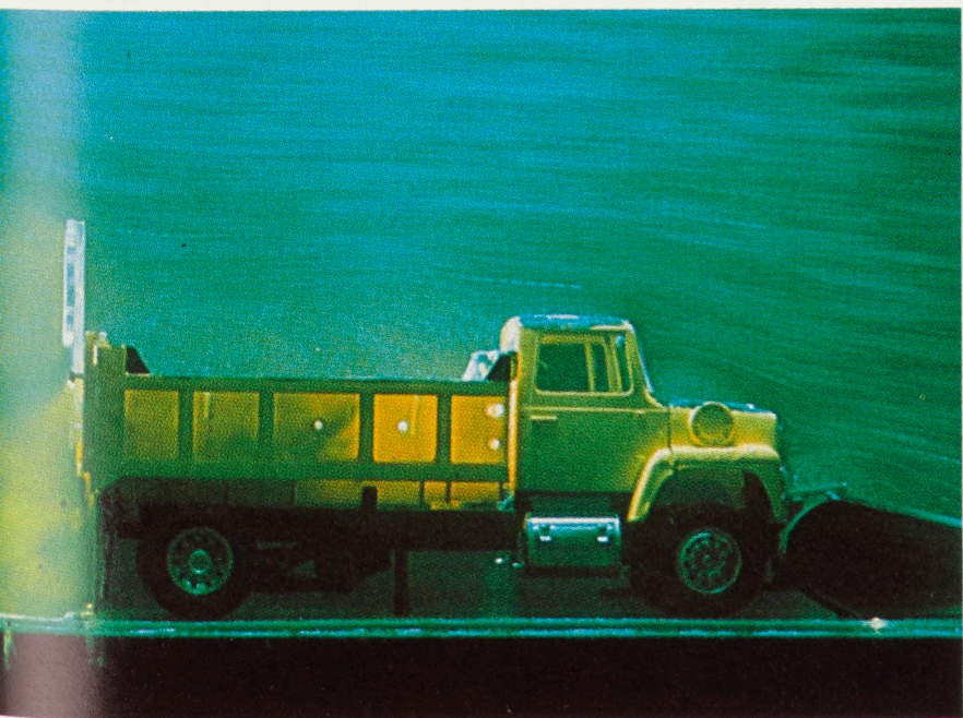
Flow patterns around a model truck mounted with a snow plough are visualized in a water tunnel. Left: the truck as normally used on the highway. Turbulence in its wake generates a mini-blizzard, dangerously obscuring vision from behind. Right: a turbulence minimizing configuration for snow ploughing, identified at the NRC and now being field tested.
