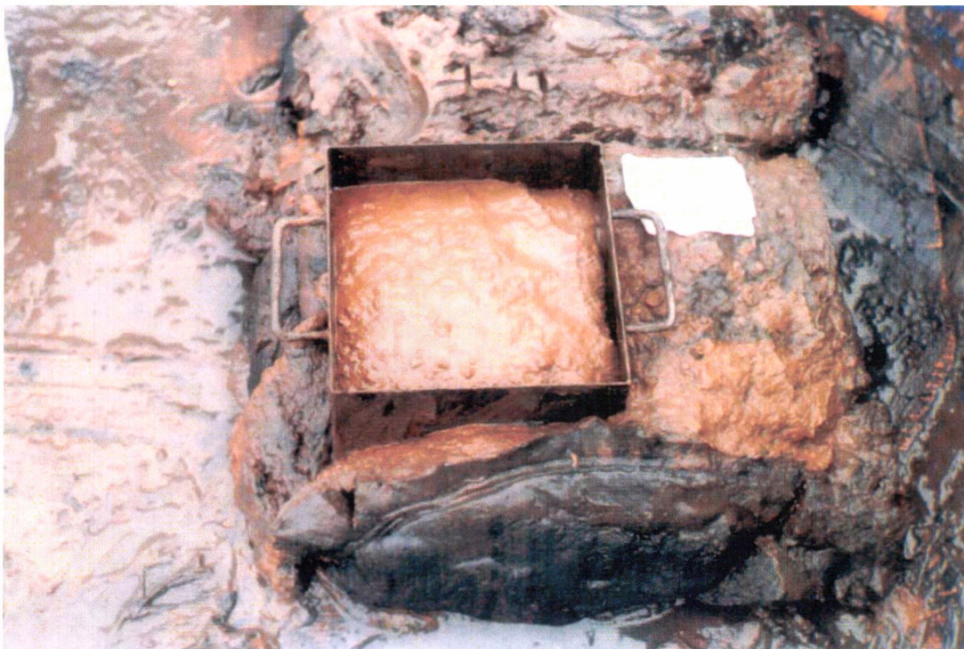
Figure 6. Square corer (0.05m 2 ) used for obtaining samples of seabed animal community July 2004.
