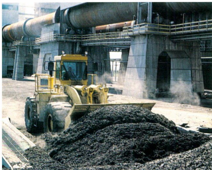
Shredded tires – demonstrating an energy source at the Lafarge Canada Inc. cement plant in Quebec.
