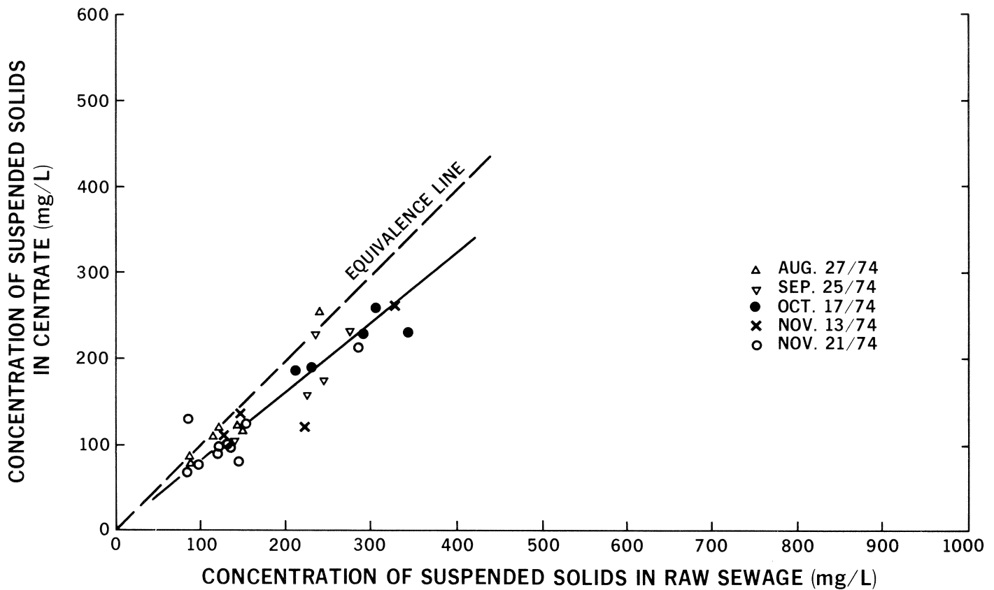
FIGURE 23. CONCENTRATIONS OF SUSPENDED SOLIDS IN RAW SEWAGE VS CONCENTRATIONS OF SUSPENDED SOLIDS IN CWC CENTRATE - NON-FIRST FLUSH CONDITIONS
