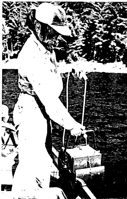
Sampling for benthos using an Ekman dredge on Lake Dorset
