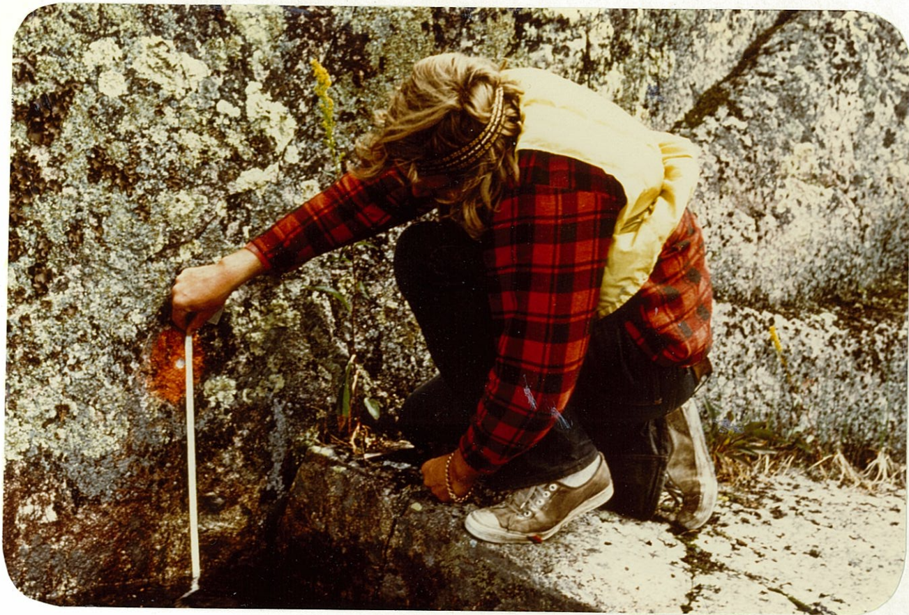
1. A typical bench mark similar to those made at all lakes as a reference point from which to measure fluctuations in water levels in future years.
