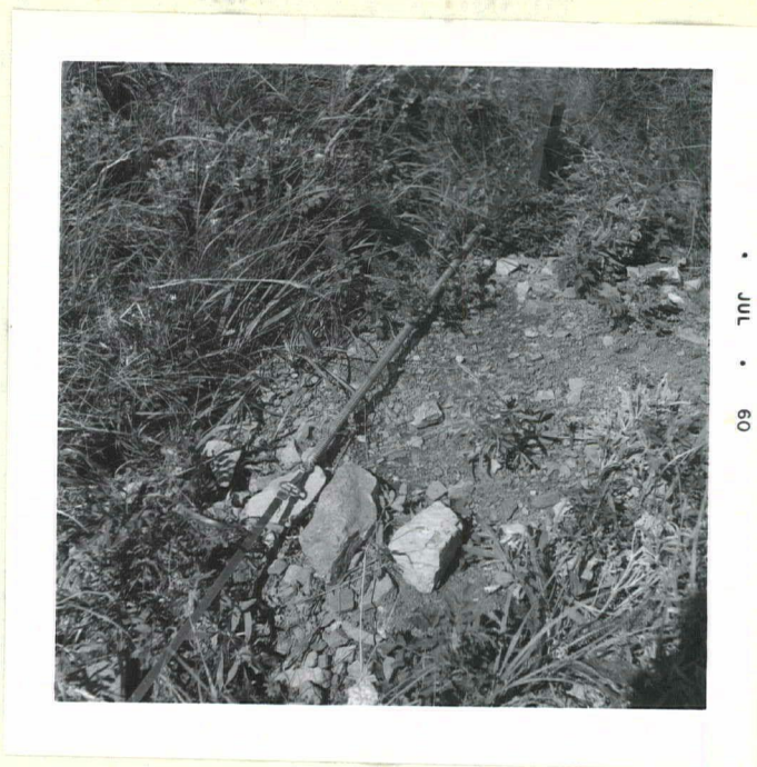
Fig. 1. Use of door spring to maintain tension on tape.
