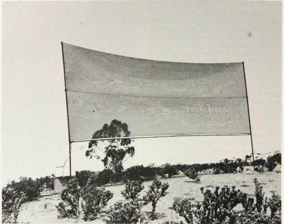
Net set up by Bob Schemenauer to collect water from fog in northern Chile
