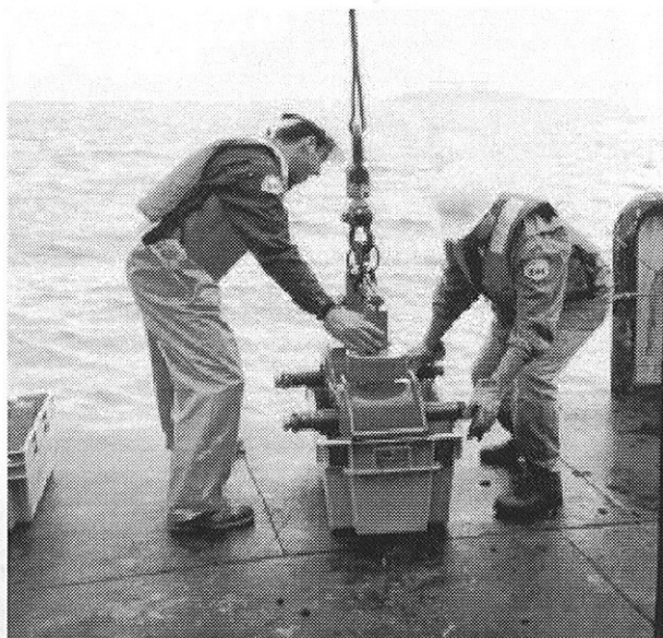
Sediment sampling using a grab sampler (Photo: Donald St-Laurent, Environment Canada).
