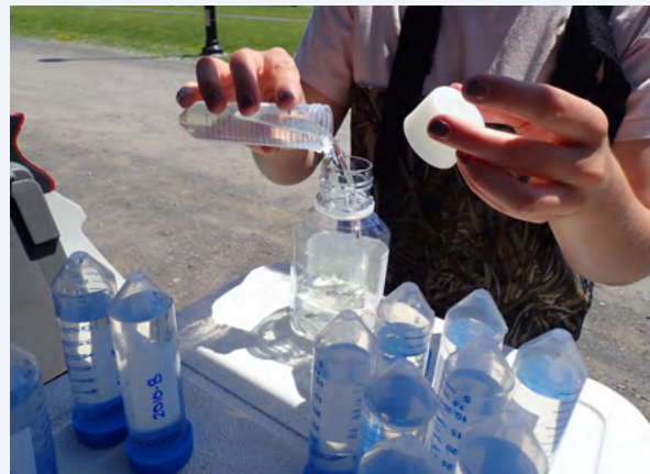
Two composite samples are prepared for each site from the various individual samples taken. Photo: Caroline Anderson, MELCCFP
