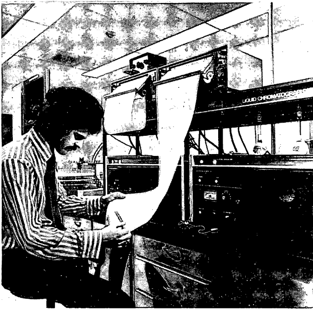
Figure 31. Richard Larose measures the peaks of a variety of separated phenols by High-Speed Liquid Chromatography.
