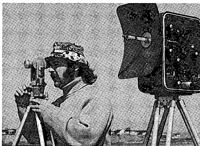
Figure 4. MRB 2 Hydrodist shore station used in range-bearing mode on Lake Huron.
