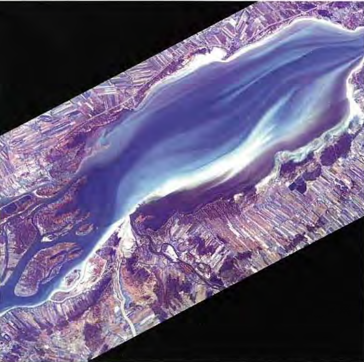
Remote sensing image showing the turbidity of water masses in Lake Saint-Pierre on October 20, 1990. The very turbid water (high suspended solids content) coming from some tributaries shows up white. The main water mass of the Great Lakes appears as dark blue, and the purple along the north shore is the Ottawa River water mass.
