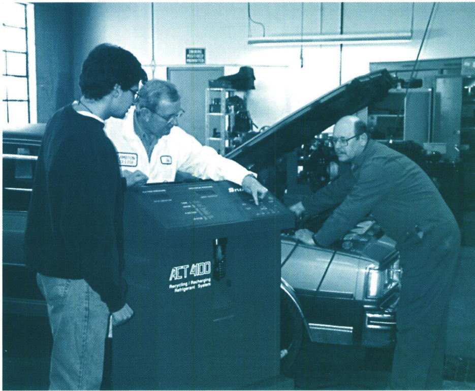
Recovery of refrigerants from automotive air conditioning.
