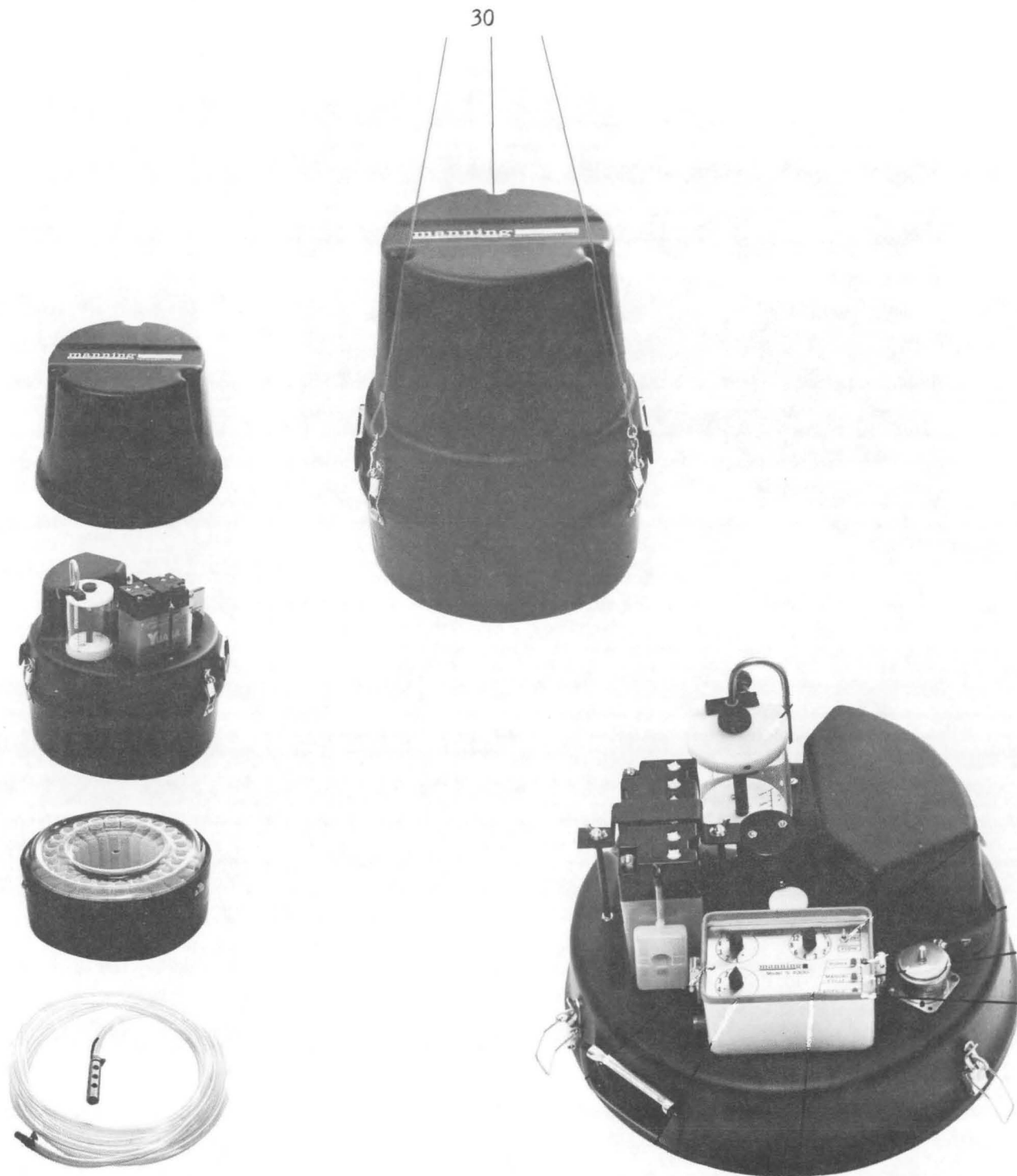
c) Sequential Sampler With Flow or Time Control Option (from Manning Environmental Corporation)
