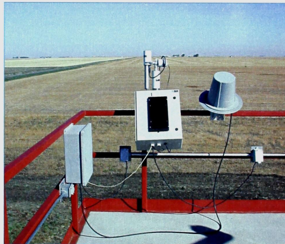
Figure 27 – Image of the Cimel sunphotometer that measures aerosol optical depth with its satellite antenna to the left by which it transmits data to NASA via the Geostationary Operational Environmental Satellite (GOES).
