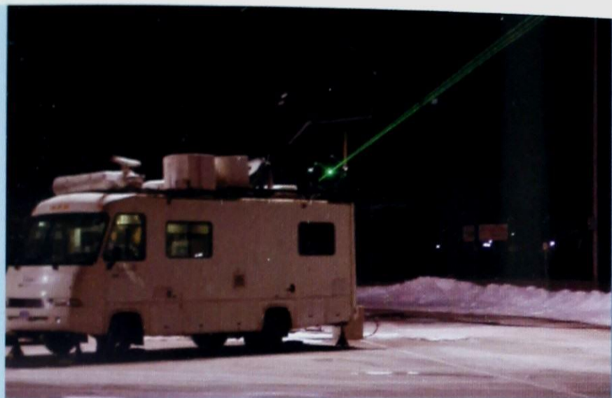
Figure 11 - RASCAL mobile laboratory in action (a laser is being projected high into the troposphere to spot pollutants in the air).
