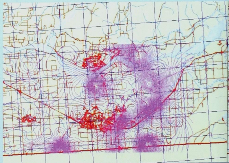
Figure 14 - Passive sampling of ambient ammonia ( \text{NH}_3 ) in the Abbotsford, B.C. area showing the impact of discrete sources.
