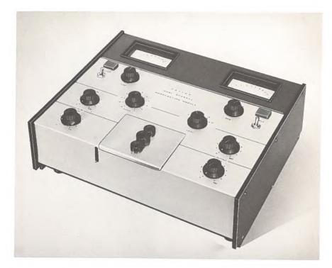
An aggregation module that permits visual study of platelet aggregation of blood plasma under controlled conditions is produced by Payton Associates Limited. The device — used to ascertain how and why platelet aggregation takes place — has proved particularly useful in studies of blood platelet reaction to certain stimuli, and platelet response to surfaces in thrombotic states.
