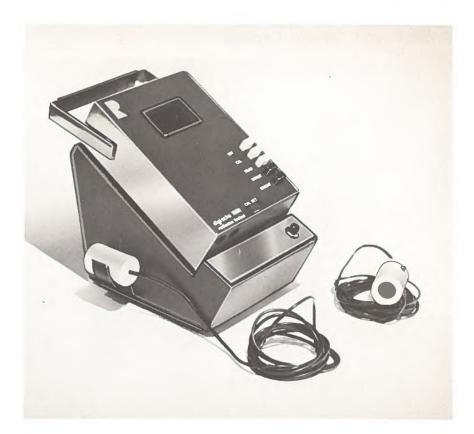
A portable, easy-to-use echoencephalograph that calculates off-center displacement and size of central brain structures is produced by Radionics Limited.
