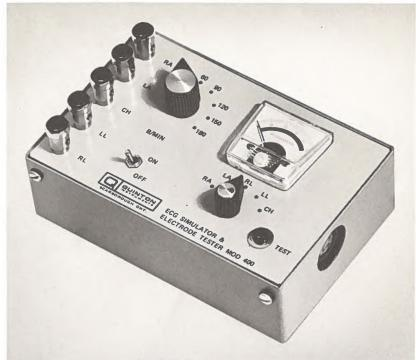
The Model 400 from Quinton Instruments Canada Limited is really two instruments in one — an ECG simulator and an electrode/skin-resistance tester.
