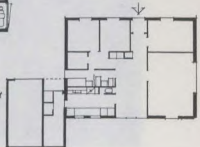
The isometric and plan show the compact arrangement of fitments in the 'heart' unit. Everything requiring plumbing is included in an area of 7ft 4in by 14ft 2in. Right, plan of a typical 'heart' house
