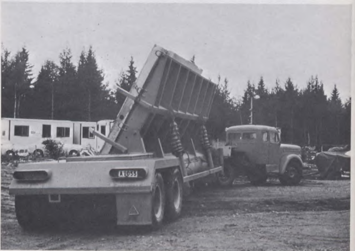
Special trucks equipped with hydraulic tilting platform.
